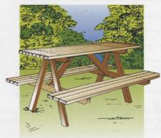
Here is a strongly constructed Bar-B-Que table and combination seats. The design has been planned so that no joints are required. The whole assembly is held together by non-corroding galvanised bolts, and countersunk head screws.
